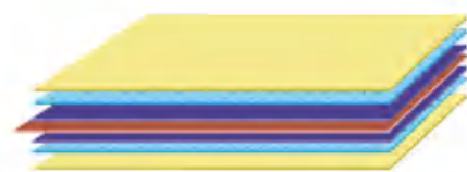
■ Lubrication layer ■ Hydrophilic coating ■ Corrosion resistant coating
